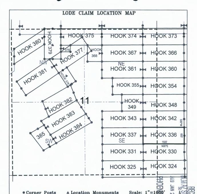
1. The above map depicts the HOOK 336 Lode Claim, which is located in the NE 1/4 of the SE 1/4 and SE 1/4 of the SE 1/4 of Section 11, and SW 4/4 of the SW 1/4 and NW 1/4 of the SW 1/4 of Section 12, Township 1 North, Range 15.5 East, Gila & Salt River Base and Meridian, Gila County,
